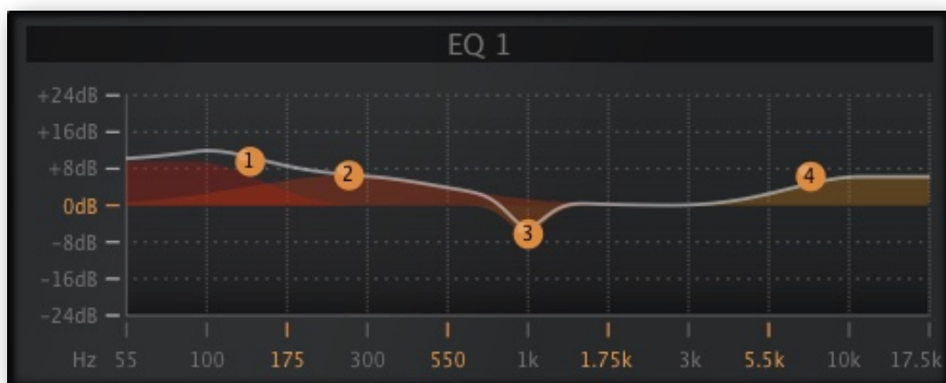
Equalizer module, bass+treble boost, dip around 1 kHz
